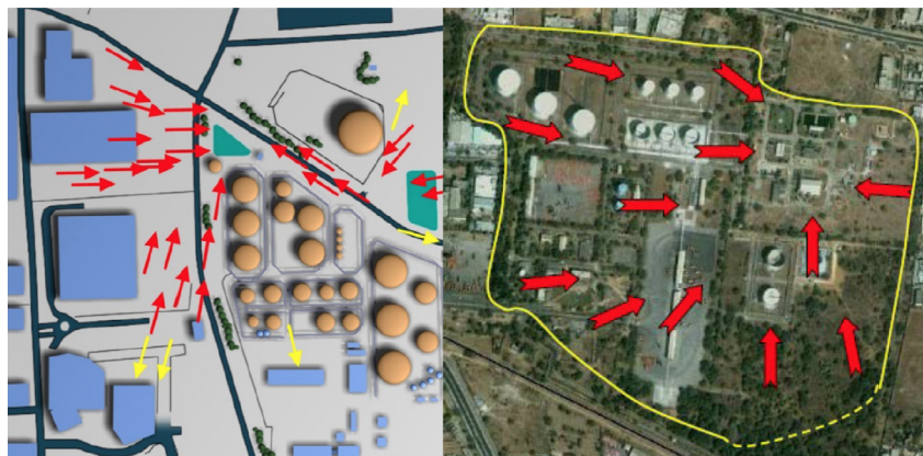
Fig. 23. Examples of directional indicators found in the detonation incidents at Buncefield (left) [1] and at Jaipur (right) [6]. The yellow boundary on Jaipur marks the edge of the vapor cloud. (For interpretation of the references to color in this figure legend, the reader is referred to the web version of this article.)
