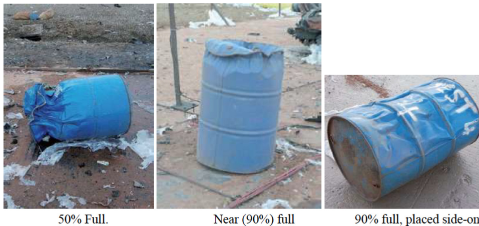
Fig. 16. Damage to standard steel oil drums placed inside the detonation, (photographs reproduced from [33,34]).
