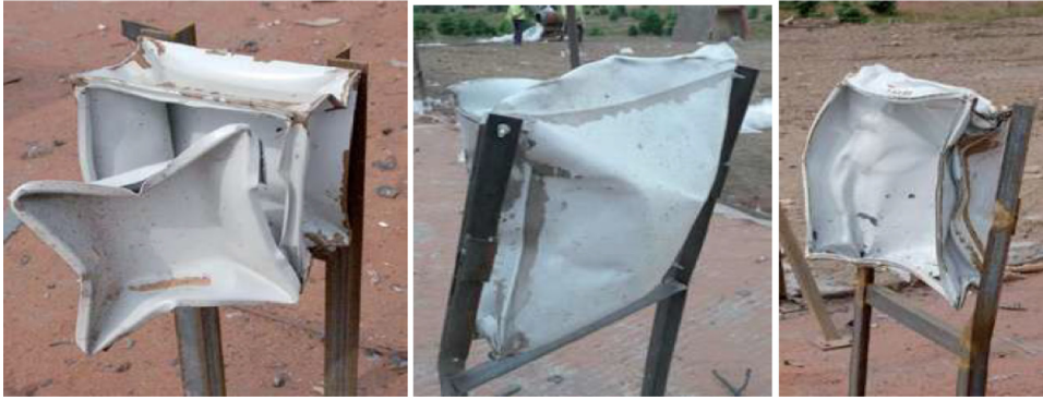
Fig. 17. Damage to small and large instrument boxes placed inside the detonation, (photographs reproduced from [33,34]). Left figure: A small box, 30 cm × 30 cm. Middle figure and right figures: Two views of a larger 60 cm × 60 cm box.
