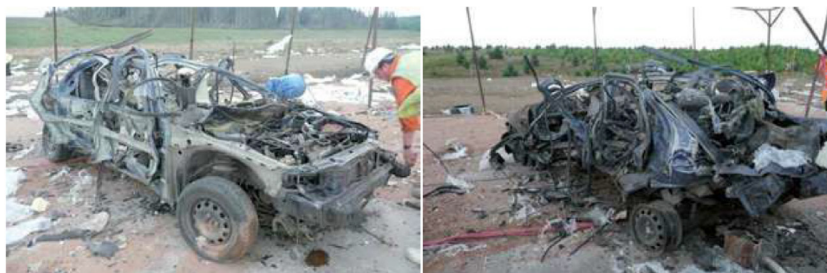
Fig. 14. Damage to cars placed inside a detonating propane-air cloud [33,34].
