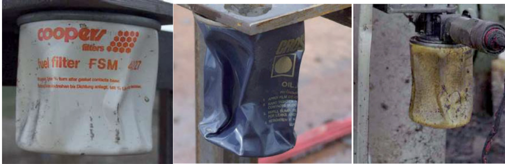
Fig. 18. Air-filled oil filters placed inside the detonation (photograph reproduced from [33,34]) compared to an oil filter recovered from the Buncefield explosion (shown on the extreme right).
